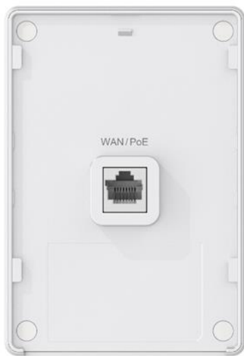
Figure 1-3 Rear View of Access Point
